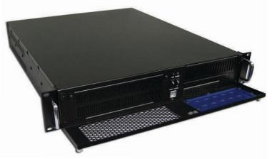
The new ICX-421-G from Captec is our most robust off-the-shelf 2U dual processor server. Harnessing the power of Intel's 2nd generation Scalable Xeon processors, this server has a number of design features that enable operation in demanding and challenging industrial environments not compatible with a typical enterprise server.
